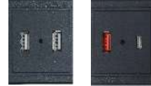
USB Port (A, A) USB Port (A, C) [Type-A; 18W, Type-C; 33/65W]
